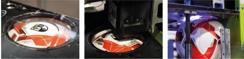
The logo is printed using an industrial UV ink jet directly on the ball surface.
